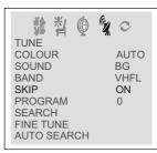
5 Press the TUNE button to close the menu. When you use the P+/buttons to select channel, this channel will be skipped. However, you can still use the PROGRAM NUMBER buttons to select the skipped channel numbers.
